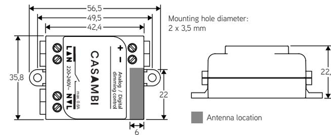
Note 1. CBU-ASD is a built-in class II device. Use double insulated wires or an external mounting box if the device is not mounted inside another insulated device.
