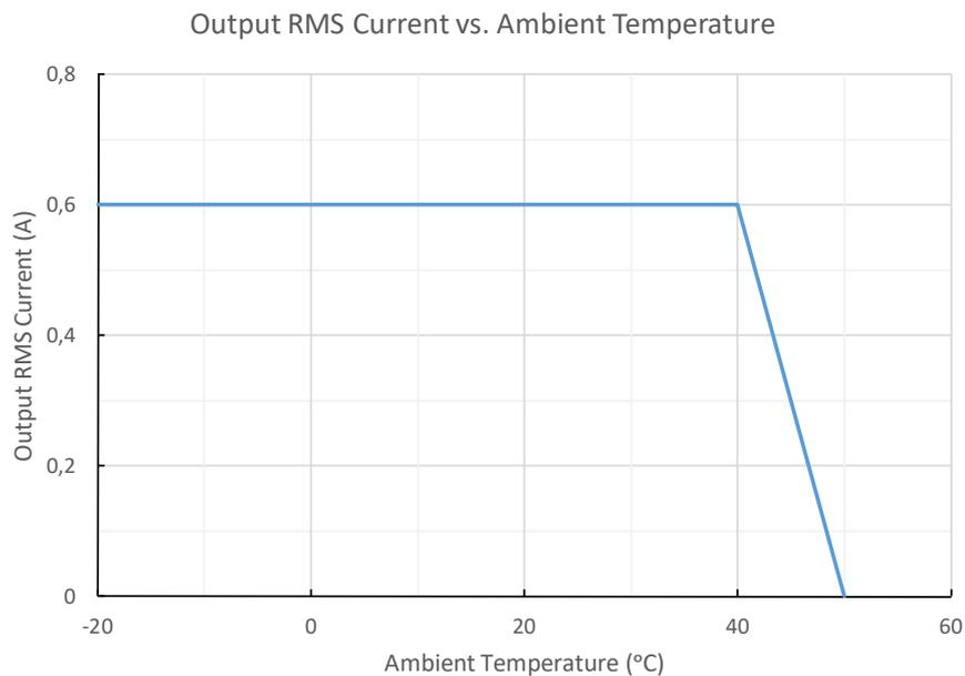
Picture 4. Output RMS current vs. ambient temperature
